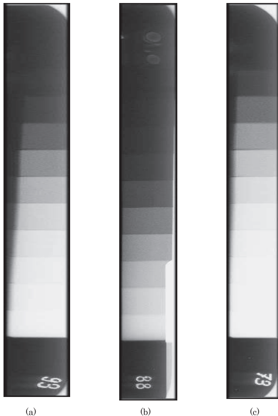
Fig. 7 Example of Step Wedge. : (a) 27kV and 31mAs. (b) 28kV and 80mAs. (c) 26kV and 22mAs
