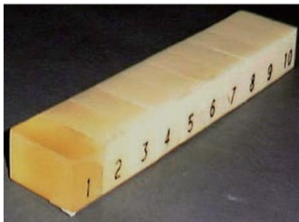
Fig. 2 Photograph of a stepwedge made from calcium phosphate with 10 steps of different densities.
